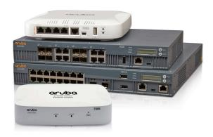
The 7000 series handles other enterprise-critical capabilities like authentication, encryption, IPv4 and IPv6 services, Adaptive Radio Management™, ClientMatch™, and RFProtect™ spectrum analysis and wireless intrusion protection.
